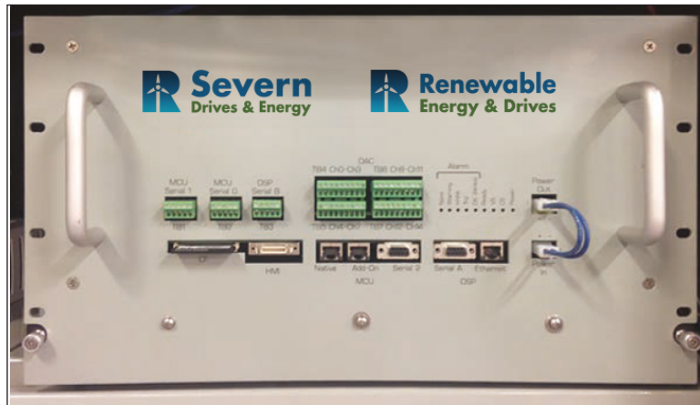
Figure 6. Control assembly inputs and indicators.
