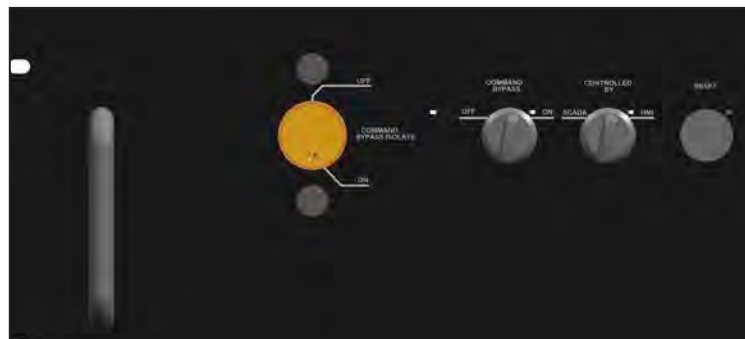
Figure 7. Master control rack control panel.
