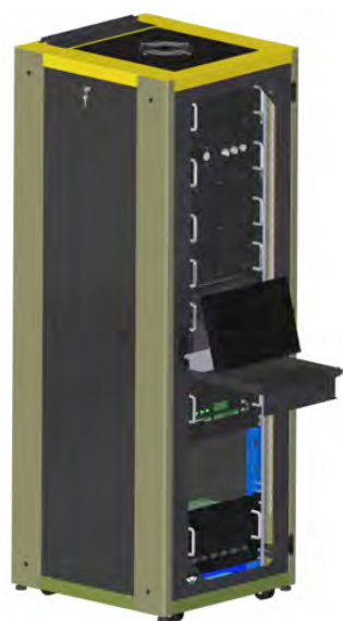
Figure 8. Master control rack with HMI screen and keyboard deployed.
